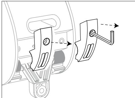
Unscrew the two fixing clamps.
