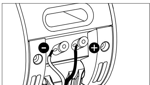
Connect the "+" from the amplifier to the "+" on the Sib (red) and the "-" from the amplifier to the "-" of the Sib (black).
