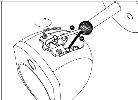
Connect the cables to the satellite speaker [taking care to observe the correct polarity] and then unscrew the machine screws using the Allen key provided.
