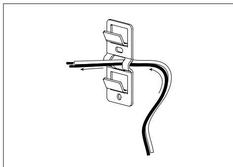
Pass the cables through the wall mounting.
