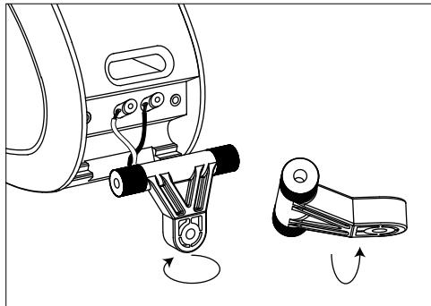
Remove the silver support piece, turn it 180°, and reposition the support so that it will fit horizontally with the wall mounted base.
