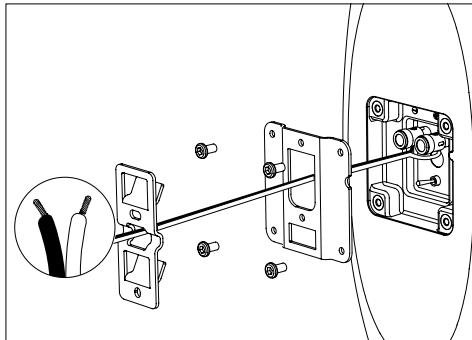
Fix the female part of the mounting to Super Bird using the screws provided and then connect the cables to its satellite speaker (taking care to observe the correct polarity).
