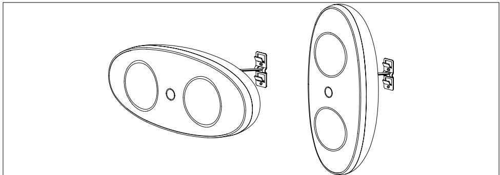
Locate the speaker onto the wall mounting. Super Bird can be mounted horizontally for central use or vertically for use as a left or right speaker.
