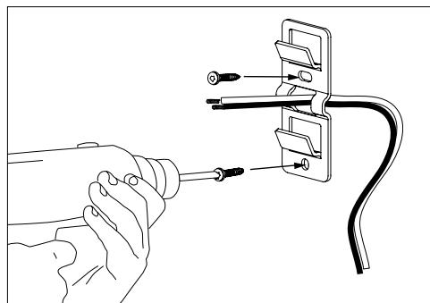
Then, after inserting the wall plugs into the wall, secure the male part of the mounting.
