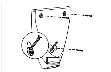
Use the base as a template to mark the position of the three fixing screws on the wall. The three fixing holes should be drilled with a Ø6mm masonry bit and the plastic wall plugs firmly inserted until they are flush with the wall surface. Fix the base with the three screws supplied.
