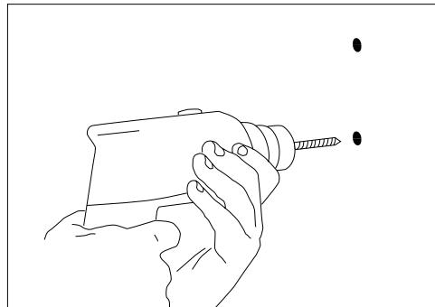
Drill the wall using the marks made previously. Insert the wall plugs in the wall.
