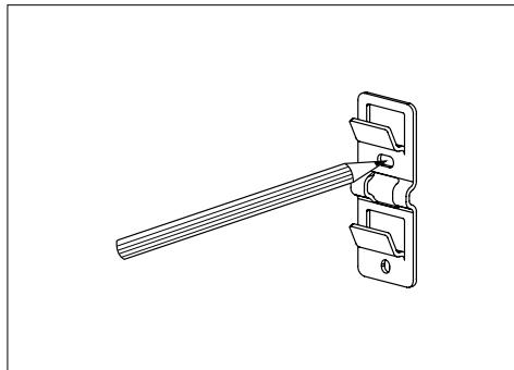
Use the male part of the fixing to fixer to the wall. Mark the locations of the fixing holes.
