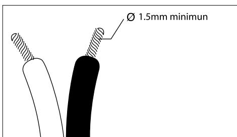
As with any performance product, Sib should be connected to the amplifier using a high quality pure copper cable of at least Ø 1.5mm.
