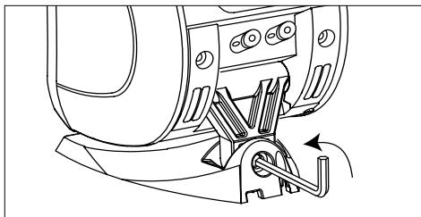
Use the hexagonal key supplied in the base of the Sib to unscrew the bolt that holds the base to the support bracket.
