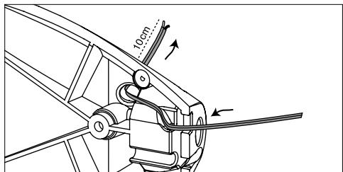
Feed the cable through the base piece as indicated in the diagram. Leave around 10cm of free cable to facilitate connection.
