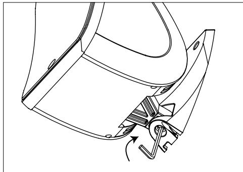
Connect up the loudspeaker cables and fix the Sib onto its wall mounted base.
